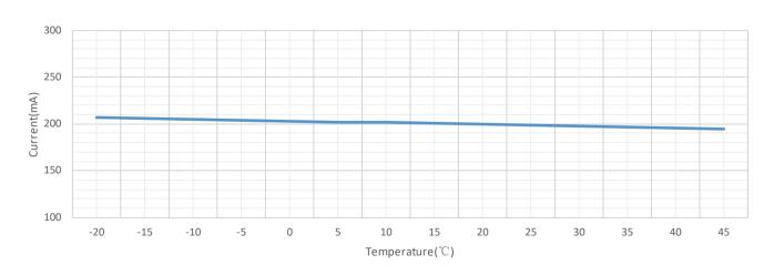
Note: This curve is test data of 1M LED Strip.
