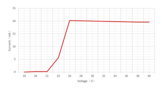
Note: This curve is tested when the IP20 1M LED Strip is under thermal stability after 2h continuous working in 15 °C room temperature.
