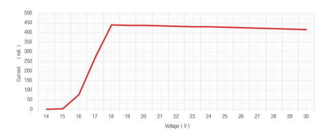
Note: This curve is tested when the IP20 1M LED Strip is under thermal stability after 2h continuous working in 15 °C room temperature.
